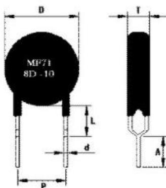
① 引线: 镀锡线 Material of Leads: Tinned Copper Wires
